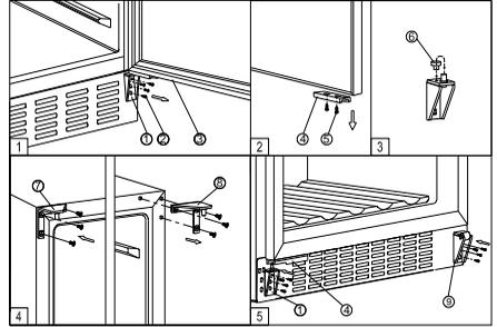
1. Remove the bottom hinge ① by unscrewing the four lock screws ②. Be careful to hold the glass door firmly after removing the screws. (Fig. 1)
