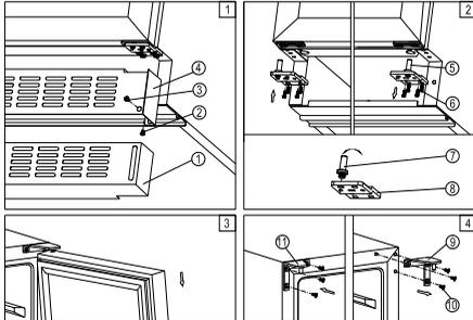
1. Remove the adjustable ventilation grille ① by unscrewing the screws ③ and then remove the ventilation grille ④ by unscrewing the screws ②. (Fig. 1)
